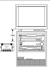
Figure 1 Connection Hub Placement
